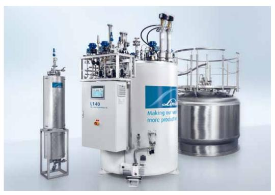
The newly developed, fully automatic computer controlled L-Series offers a wide range of liquefaction and refrigeration capacities, depending on liquid nitrogen ( $LN_2$ ) pre-cooling and on the chosen size of compressor. All standard coldboxes are equipped with a  $LN_2$  pre-cooling facility, which allows a significant increase in capacity. The L140/LR140 therefore provides a high degree of flexibility to meet your requirements today and in the future.
